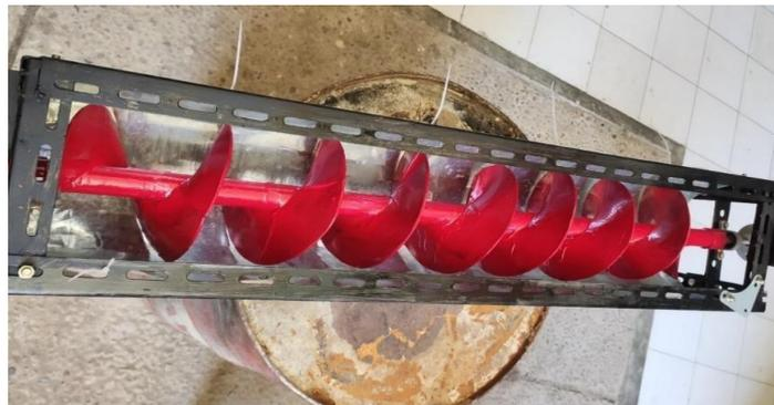
Gambar 10. Hasil Rangka Turbin Archimedes Screw
