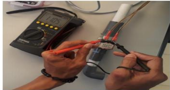
Gambar 3. Tegangan Solenoid Valve saat ON
