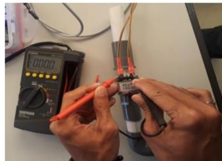
Gambar 4. Tegangan Solenoid Valve saat Off
