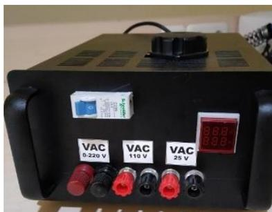
Gambar .7 Regulator Tegangan AC 1 Fasa
