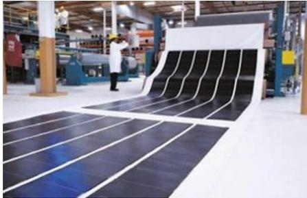
Gambar 5. PV Thin Film Solar Cell [16]
