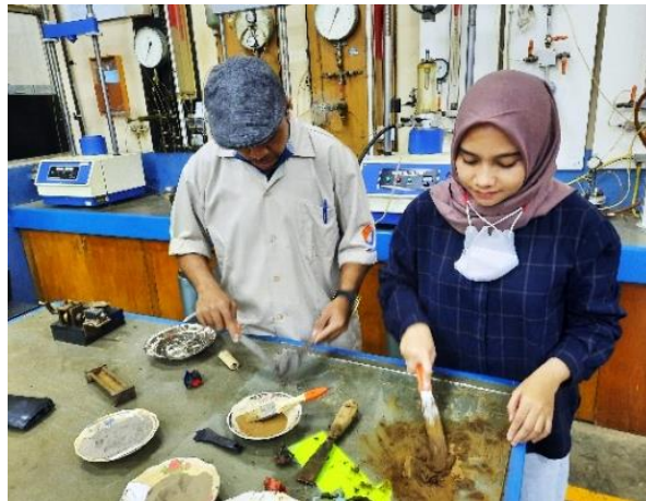
Gambar 5. Pengujian Atterberg Limits
