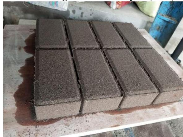
**Gambar 2b. Paving Block 10% Cocopeat (Riset, 2023)**
