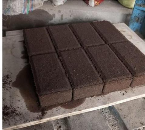
**Gambar 2d. Paving Block 50% Cocopeat(Riset, 2023)**
