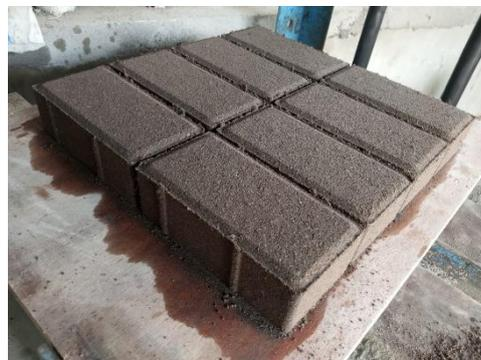
**Gambar 2c. Paving Block 25% Cocopeat (Riset, 2023)**
