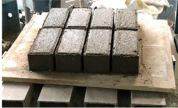
**Gambar 2a. Paving Block 0% Cocopeat (Riset, 2023)**
