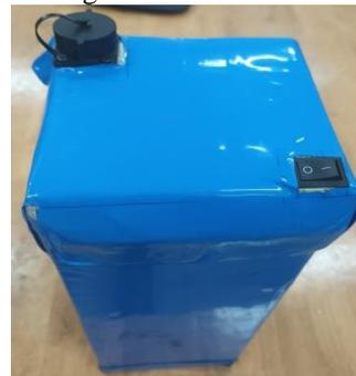
Gambar 10. Hasil Akhir Battery Pack 72V 20Ah
